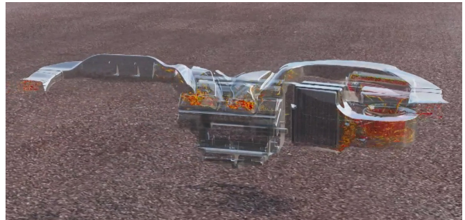
Turbulent flow structures in the 7 series HVAC.
