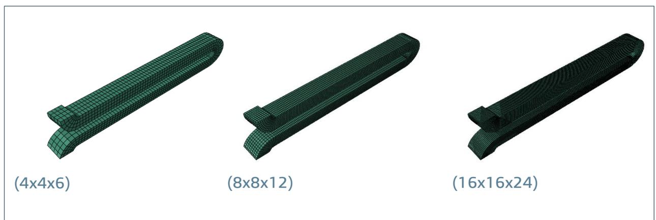
Fig 3.5: Mesh refinement levels
